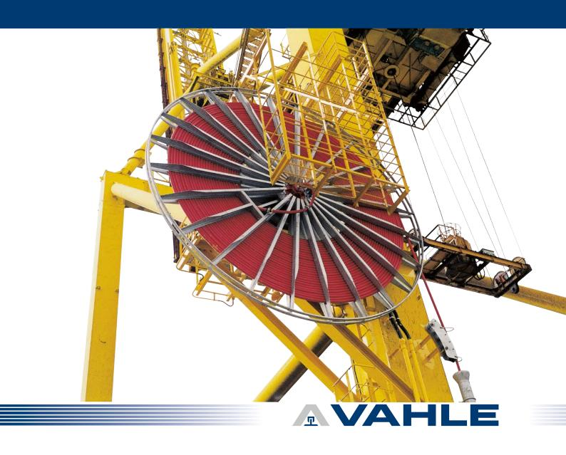
Motor Powered Cable Reels
